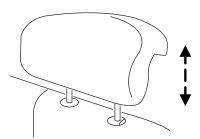
Push button to lower head restraint.
